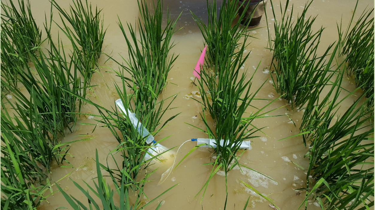
A continuously flooded rice field at Stuttgart, AR showing the setup of pore water samplers to collect soil pore water samples from the root zone throughout the field season.
